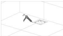
10. Filled silicone between floor drain and ceramic
